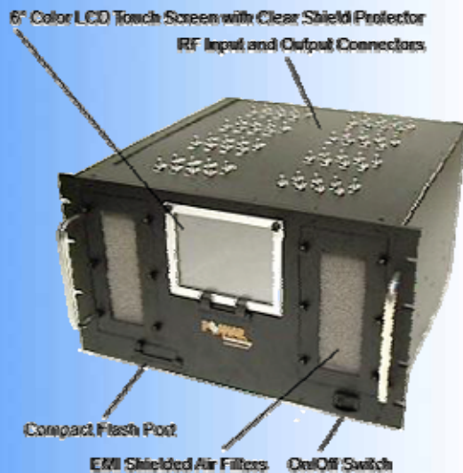
Fig.1 Front view of the PET-VI System Platform
