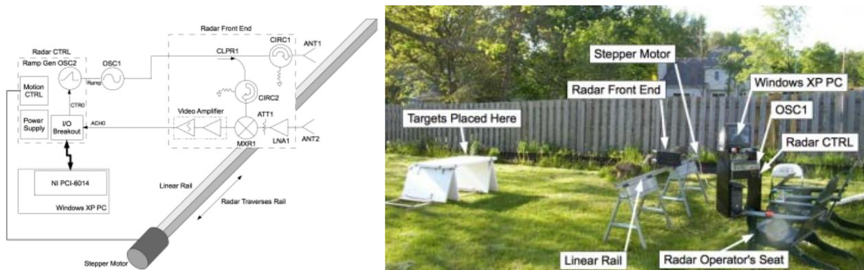
Figure 3. X-band Synthetic Aperture Radar (SAR) mounted on 8' long linear stage. .
