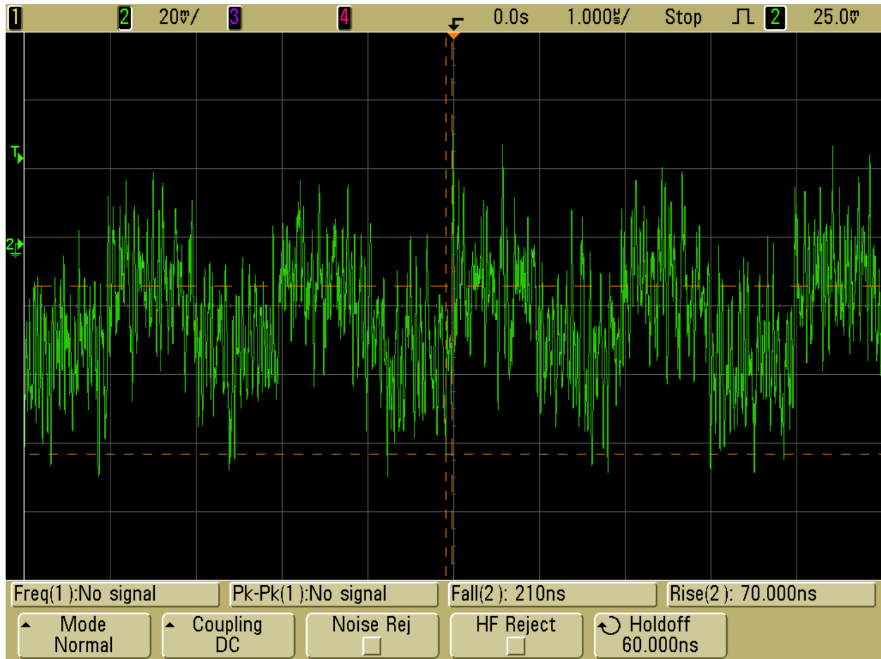
Channel 1: RF Power through Crystal Detector (Negative Voltage when power is on)
